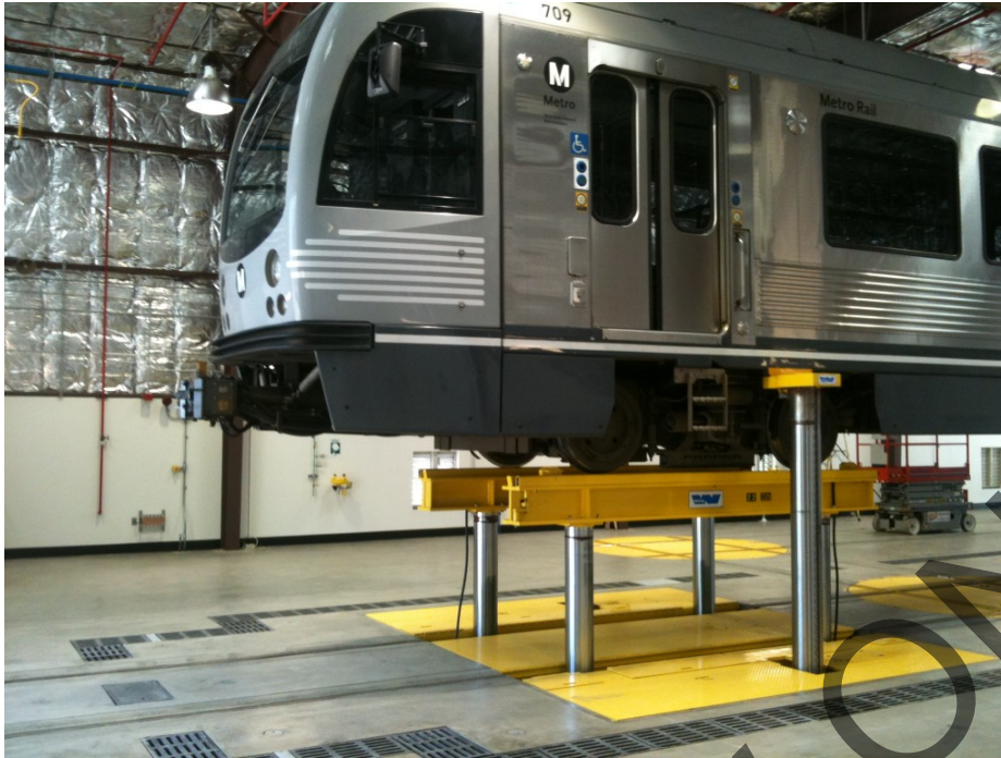
Figure 1.11 LA Metro Rail Car on Hoists –from whitingcorp.com
